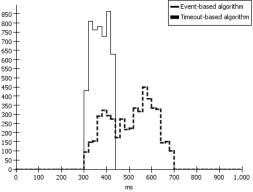
Figure 5. Difference in transition time distribution in case of timeout-based and event-based DL
