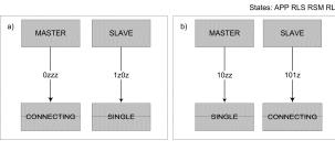
Figure 3. Transitions, which occure during failure conditions. a) MasterFailure, b) LinkFailure
