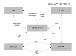
Figure 2. States and transitions of SM. Vector parameters are: APP- application state, RLS – redundant link state, RSM – state of the remote SM, RL – state of the reserved link, 'z' means 'any value'.
